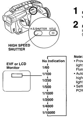
Press HIGH SPEED SHUTTER while recording.
