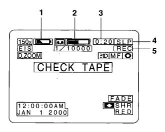
1 Battery Remaining (page 43) "WARNING LOW BATTERY" appears and Power Lamp starts flashing 15 seconds before Camcorder shutoff.
